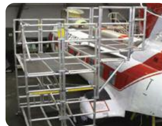
Rotor Access Stand with cantilever for commercial CH-46 Sea Knight Helicopter
